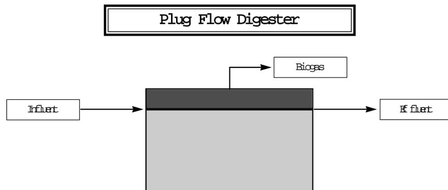
An new variation on the plug-flow digester is the slurry digester, which uses either a silo shaped reactor or a loop or horseshoe configuration. These digesters can treat a variety of animal manures and can operate at lower solids
